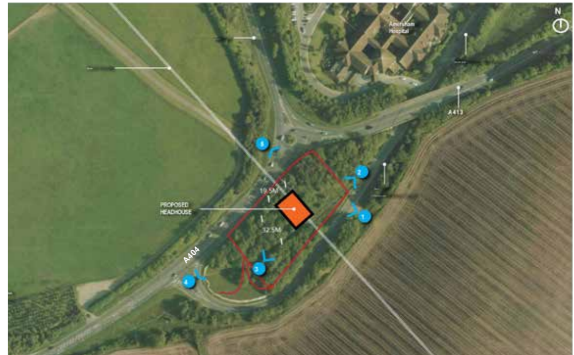
Extract from HS2 Study: Aerial photograph with building and compound overlay, Amersham (Act Limits extend to kerb line of adjacent roads)
