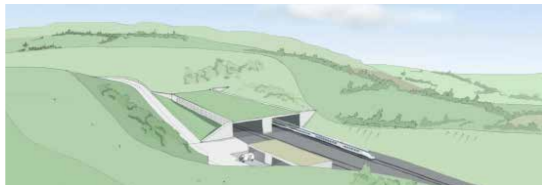
HS2 typical porous portal (illustration from HS2 Info Paper D2)
